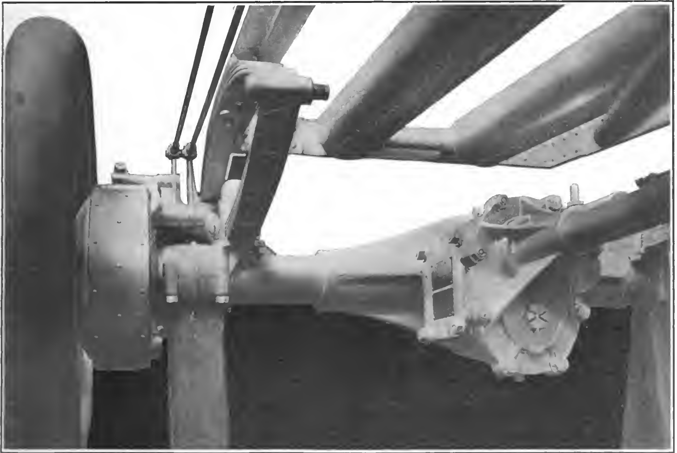
VIEW OF THE NORTHERN REAR AXLE FROM UNDERNEATH THE CAR FRAME. NOTE GEARBOX ON BACK AXLE CONTAINING CHANGE SPEED AND BEVEL GEARS, AND DIFFERENTIAL. ALSO NOTE WIDTH OF BRAKE FACE AND DOUBLE BARREL MUFFLER.
